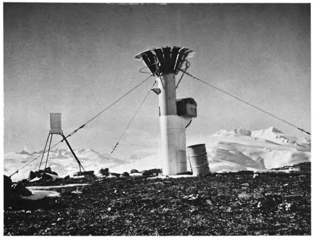
FIGURE 5.—Photograph of precipitation and air-temperature gage at Wolverine Glacier, Kenai Mountains, Alaska. This recording gage operates throughout the year at site 3, 1,000-m altitude (see pl. 3A for location). A specially designed antifreeze solution which is self-mixing enables precipitation occurring as snow to be recorded without the addition of heat. The wind screen on the left contains the air temperature sensing element.
